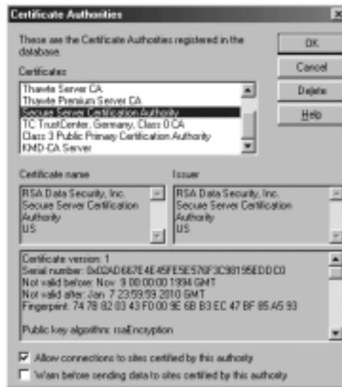
Figure 4.12 ► Commercial Web browsers are preconfigured with a list of trusted certificate authorities.
